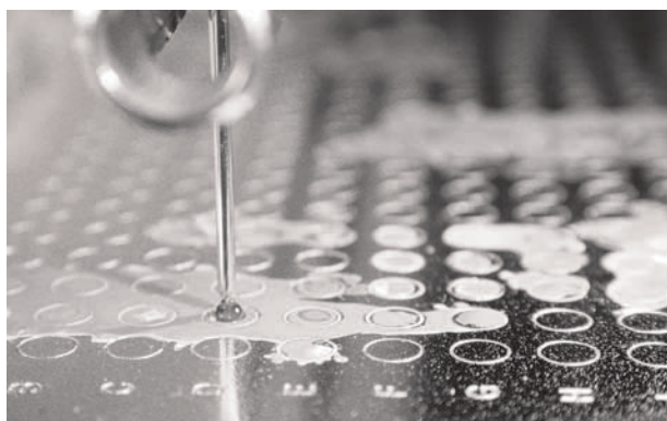
Fig 3. Direct deposition to MALDI target.
